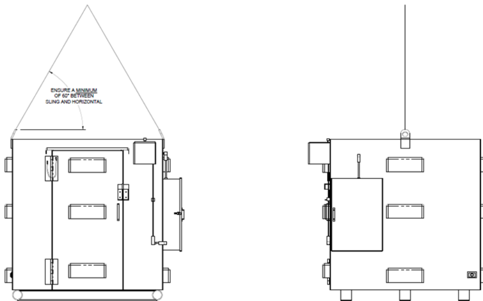
Figure 3. Typical lifting arrangement.
