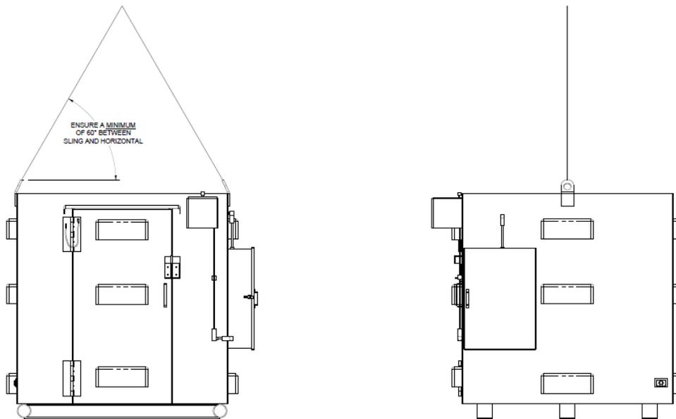
**Figure 3.** Typical lifting arrangement.
