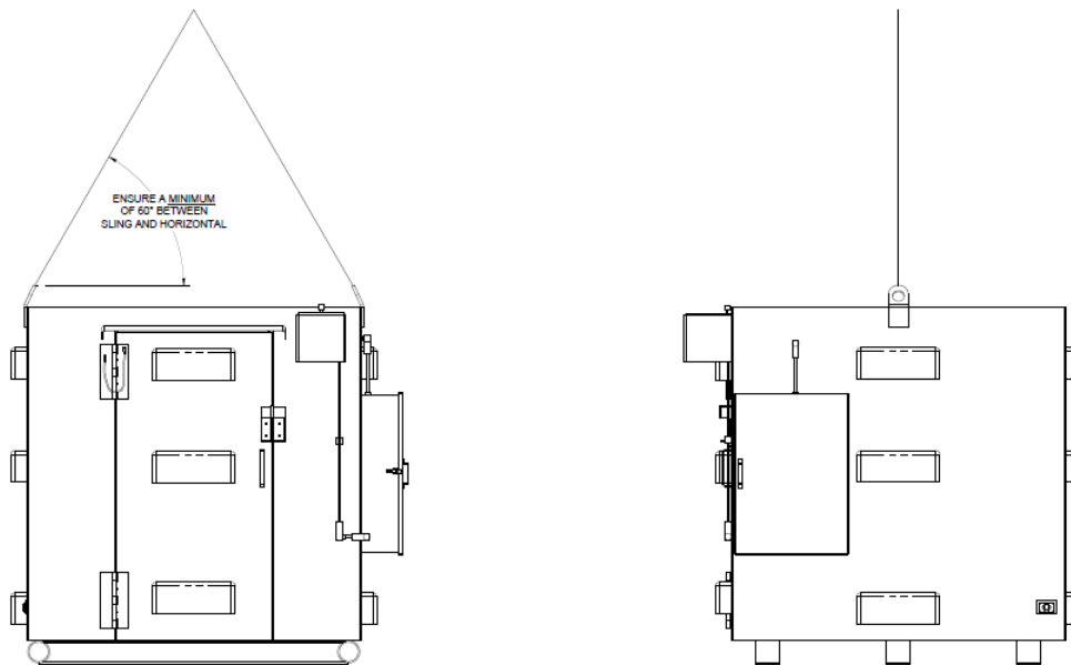
Figure 3. Typical lifting arrangement.
